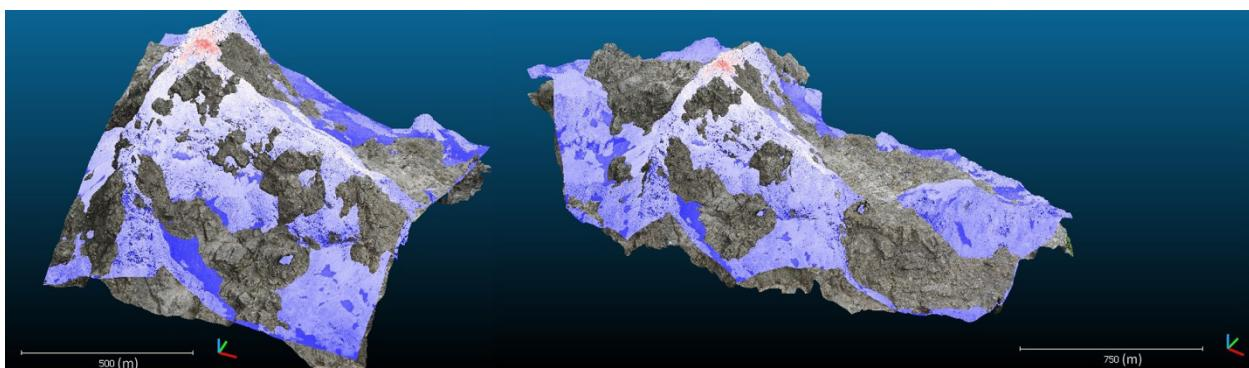
**Fig. 11** Comparison of the transformed stone model point cloud (natural colour) and the actual mountain point cloud (artificial colour), for the central area and entire area.
