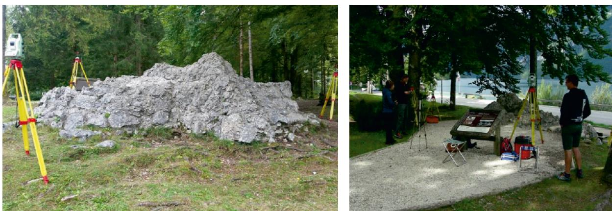
**Fig. 4** Terrestrial laser scanning of the stone model with the Leica Nova MS50 instrument
