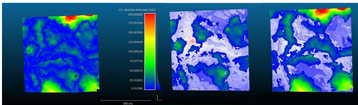
**Fig. 13** Central area, using the ICP: absolute distances, deviation of the stone-built model above the actual mountain, deviation of the stone-built model below the actual mountain.
