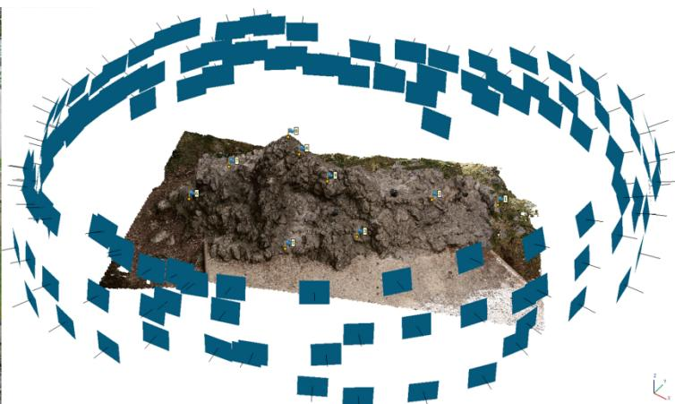
**Fig. 5** Photographing the model; point cloud with reference points and space distribution of photos taken around the model.
