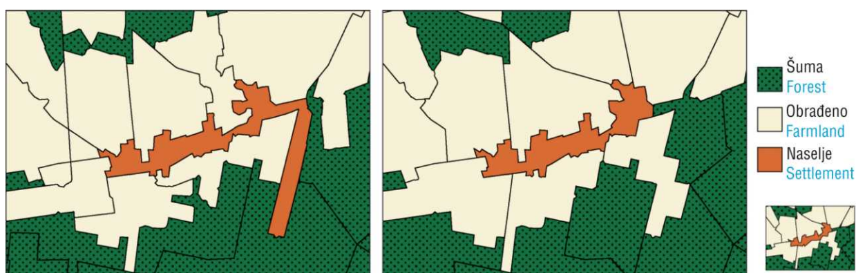
Fig. 15 Aggregation of polygonal features using the optimisation approach: (left) result with minimal class change; (middle) considering class change and compactness; (right) at a scale of 1:250,000 (adapted from Haurert and Wolff, 2010)
