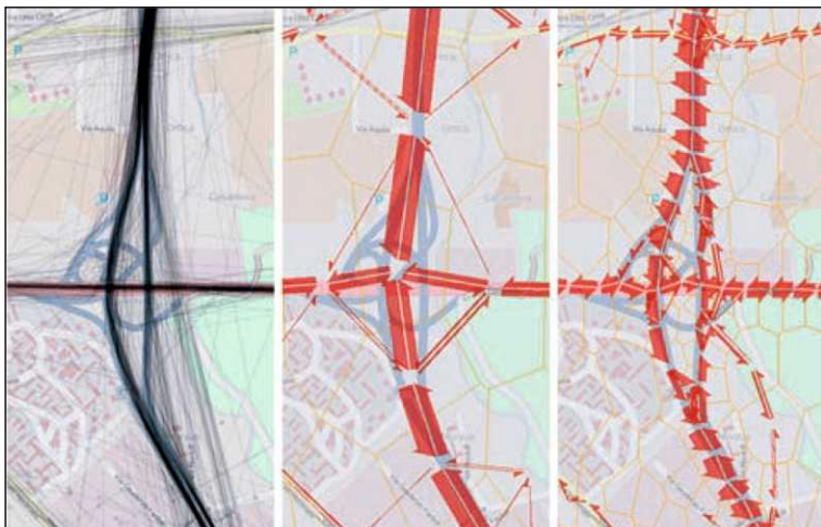
Fig. 7 Original trajectories (left) aggregated by parameters of 500 metres (middle) and 100 metres (right) (Andrienko and Andrienko, 2011) Slika 7. Izvorne trajektorije (lijevo) sažete s parametrima 500 metara (sredina) i 100 metara (desno) (Andrienko i Andrienko, 2011)
