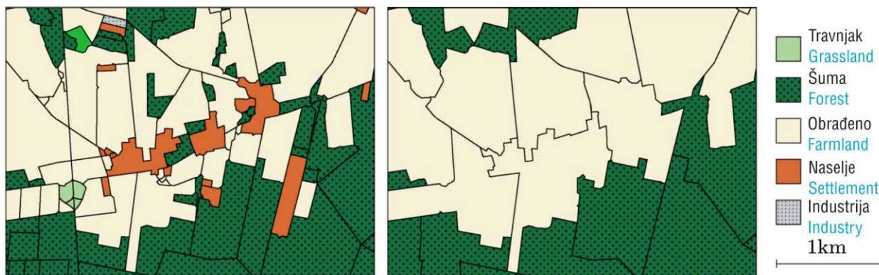
Fig. 14 Simple algorithm for the aggregation of adjacent polygonal features: (left) input; (right) result (adapted from Haurert and Wolff, 2010)
