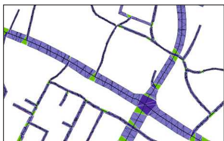
Fig. 9 Aggregation of double-lines into single lines by conversion into polygons and Delaunay triangulation (Wang and Doihara, 2004)
