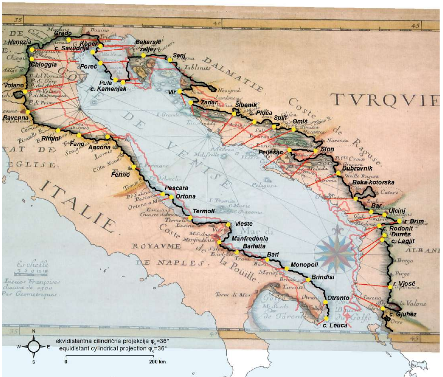
Fig. 1 Residual vectors (red) of identical points (yellow) for Pierre Duval's 1664 map, georeferenced by using the coordinates extracted from the map and with the application of its proprietary E–W shift ( \Delta\lambda_0 ). The thick black line represents its vectorized coastline, while the thick semi-transparent red line represents its vectorized coastline generated upon its geometrical best-fit.
