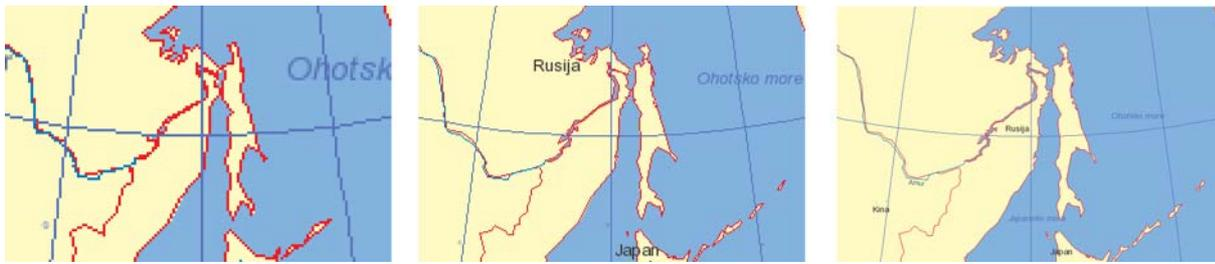
Fig. 6. The effect of line simplification with tolerance value dependent on the map scale; the original scales are: 40 000 000 (left, image enlarged 4 times), 1:20 000 000 (centre, image enlarged 2 times) and 1:10 000 000 (right)
