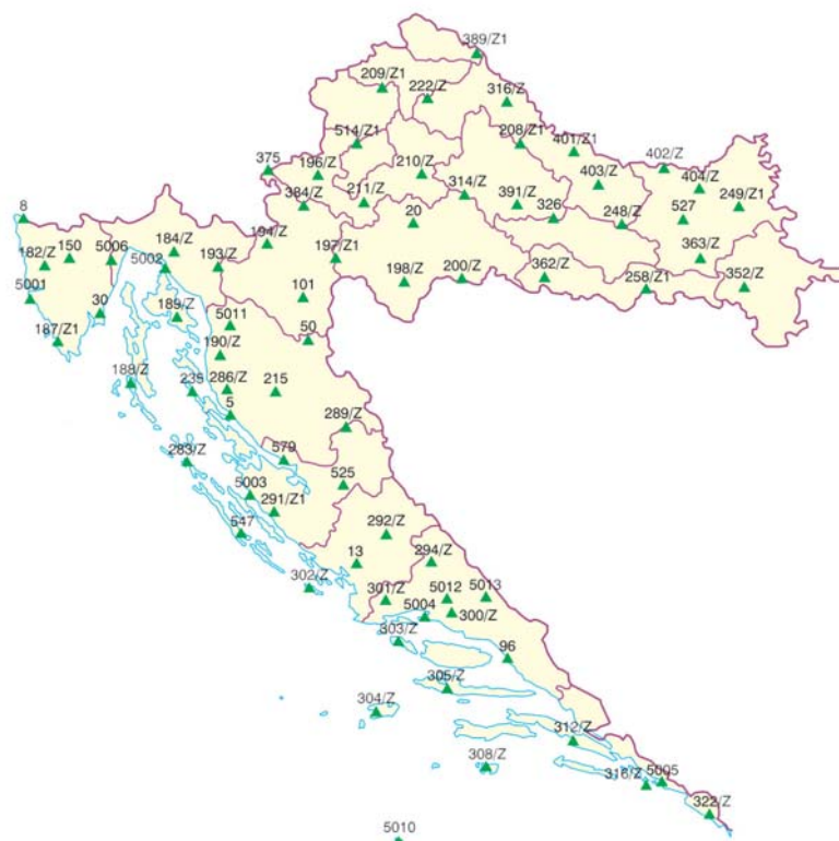
Fig. 4. Distribution of 78 basic points of positional reference frame of the Republic of Croatia
