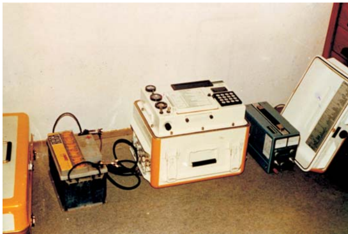
Fig. 20. (upper left) Magnavox Doppler device with accumulator at the Hvar Observatory in the IDOC'82 campaign
