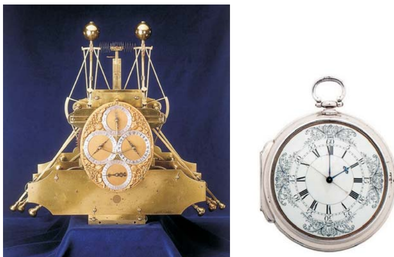
Fig. 3. H1 - the first model of Harrison's chronometer from 1735 had 33 kg (left) and H4 - the fourth version of Harrison's chronometer from 1761 (right). A duplicate of that model was produced by Larcum Kendall, and used by J. Cook on his second journey from 1772 to 1775 (URL 10)
