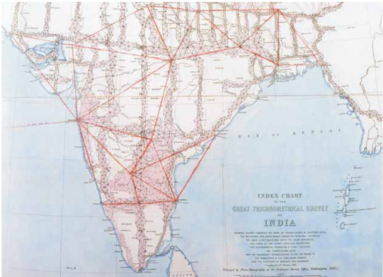
Fig. 18. Map showing triangulation links for the Great Trigonometric Survey of India of 1880, on the basis of which the height of the Himalayan peaks was determined, and Mt. Everest discovered to be the highest peak in the world (by permission of the Royal Geographical Society (with IBG))
