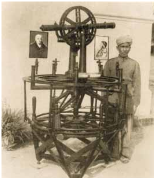
Fig. 12. Lambton's huge theodolite, having 500 kg (by permission of the Royal Geographical Society (with IBG))
